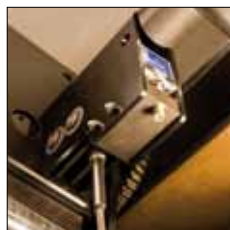
Overload prevention device prevents lifting excessive loads
