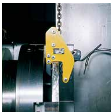
Special version of universal grab model TAG with modified side plates for use in confined spaces.
